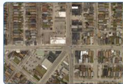
Large swaths of asphalt in commercial areas can spill concentrated heat into surrounding residential areas that lack protective vegetative buffers.
